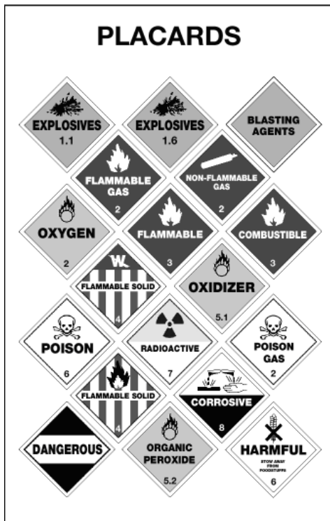
Figure 29: Hazardous Material Placards
