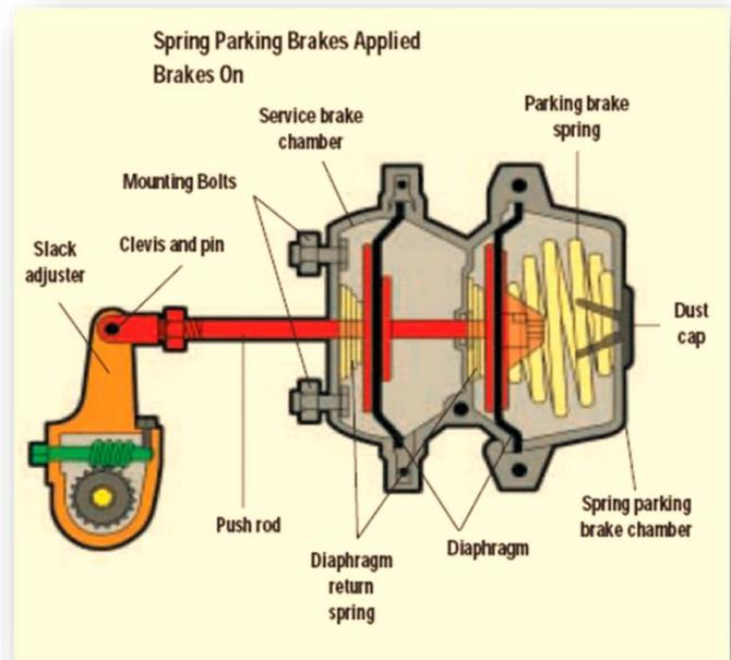
A parking brake control in the cab allows the driver to let the air out of the brake chamber, which results in the spring applying the brakes (the linings will be forced against the drums). A leak in the air brake system, which causes all the air to be lost, will also cause the springs to put on the brakes.
