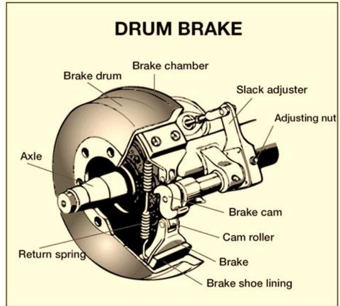
Figure 5.2 Drum Brake
