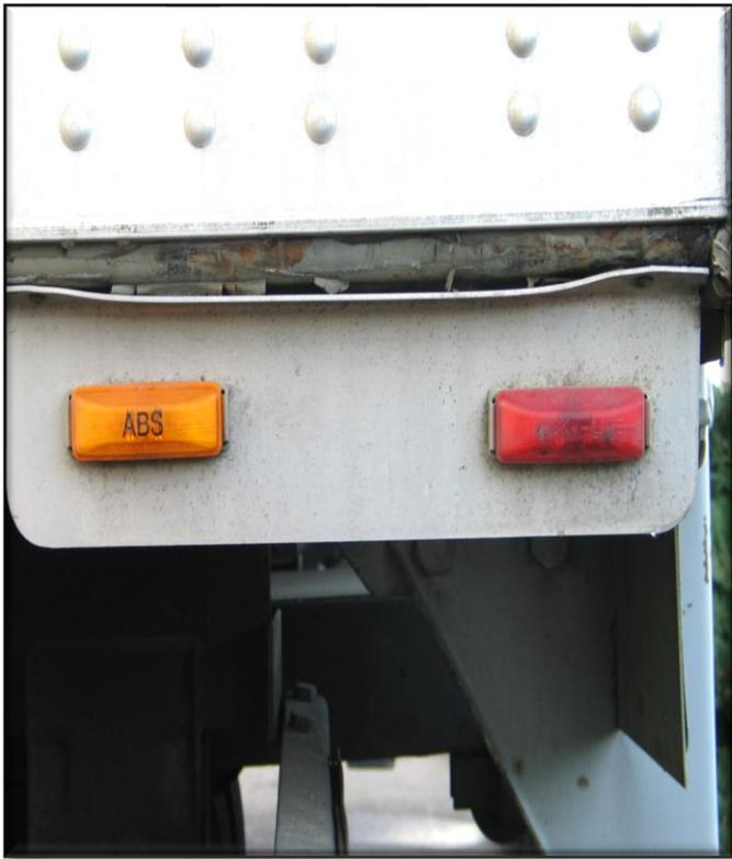
**Figure 6.7 – ABS Malfunction warning Light.**
