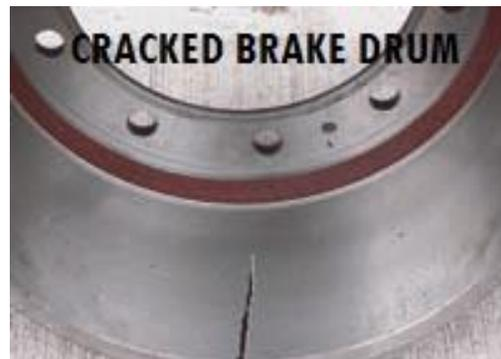
Cracked drums or rotors may lead to loss of brake response. Worn drums or rotors can cause excessive heat buildup from reduced ability to absorb and dissipate heat or possible “CAM OVER” of S-cam brakes.
