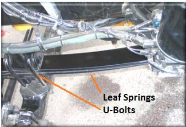
**Spring Mounts:** Consist of the brackets, bolts, shackles, and bushings used for attaching springs and/or air bags to vehicle frame. Loose, worn, or broken components may lead to loss of vehicle control or rollover.
