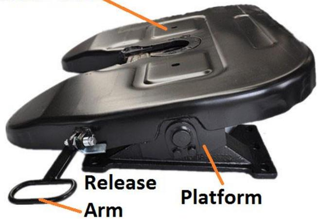
**Release Arm (Fifth Wheel)** releases fifth wheel locking jaws so that the trailer can be uncoupled. The release arm must be in the **engaged** position with locking jaws completely closed around the kingpin when pulling a trailer. This will prevent loss of the trailer during travel.
