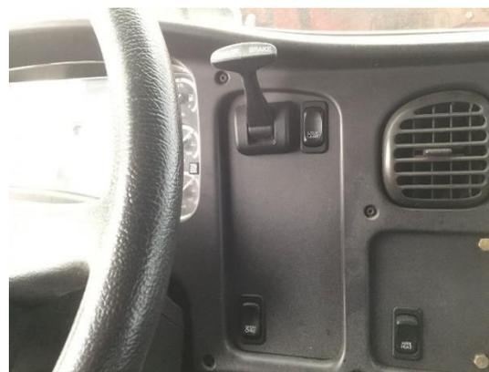
**Trailer Brake Handle in Freightliner Tractor**
