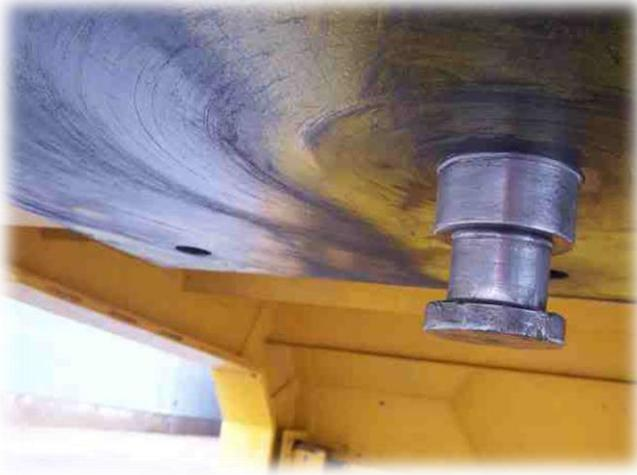
**Fifth Wheel Gap:** When coupled, there should be no visible gap between the fifth wheel surface and the trailer apron. If there is a gap between the face of the fifth wheel (skid plate) and the metal kingpin plate (apron) of the trailer, the trailer is not coupled correctly and could result in the loss of the trailer during travel.
