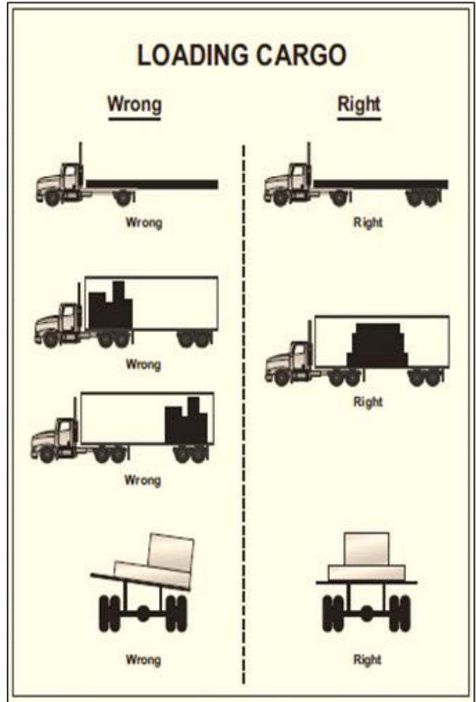
**Figure 3.1 Loading Cargo Correctly**
