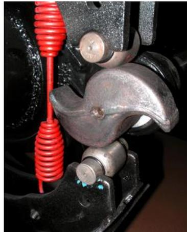
Air pressure pushes the rod out, moving the slack adjuster, thus twisting the brake camshaft. This turns the S-cam (so called because it is shaped like the letter "S"). The S-cam forces the brake shoes away from one another and presses them against the
