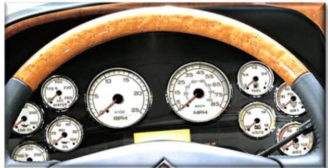
**Oil Pressure Gauge:** As soon as the vehicle is started, check the oil pressure gauge to make sure the engine has oil pressure. Too little pressure can ruin the engine.
