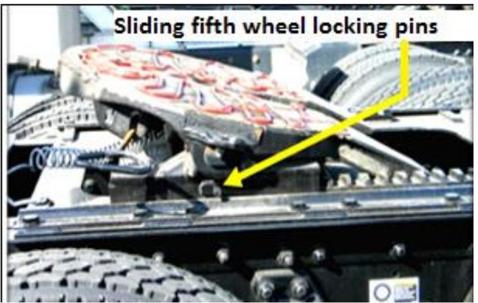
**Mounting Bolts:** Hold the fifth wheel to the tractor frame. Loose or missing bolts may cause movement between the frame and the coupling assembly resulting in handling and stability problems in turn and curves. Loose bolts could break off, resulting in loss of the trailer.
