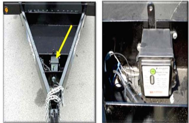
**Locking Mechanism:** The locking system on a ball hitch would be the lock that keeps the hitch locked over the ball. On a pintle hook, the locking system would be the part that locks the drawbar eye into the pintle hook.
