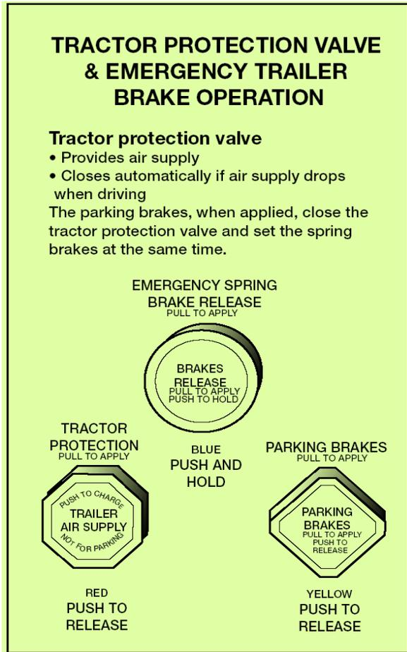
**Figure 5.3 TPV and Brake Operation**
