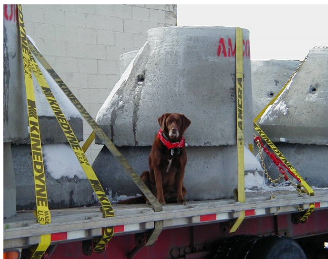
Figure 3.2 Tie Down Devices
