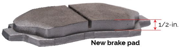
New brake pad versus worn brake pad
