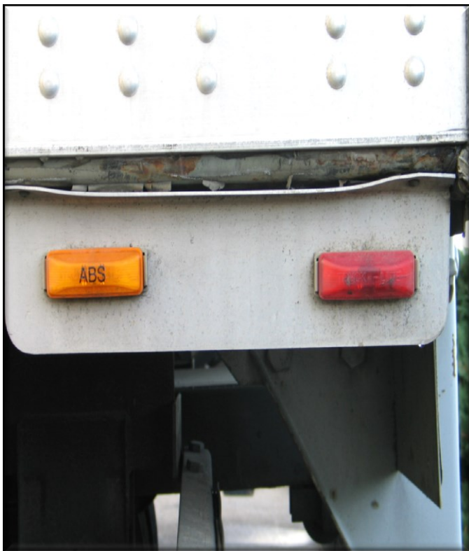
Figure 6.7 – ABS Malfunction warning Light.
