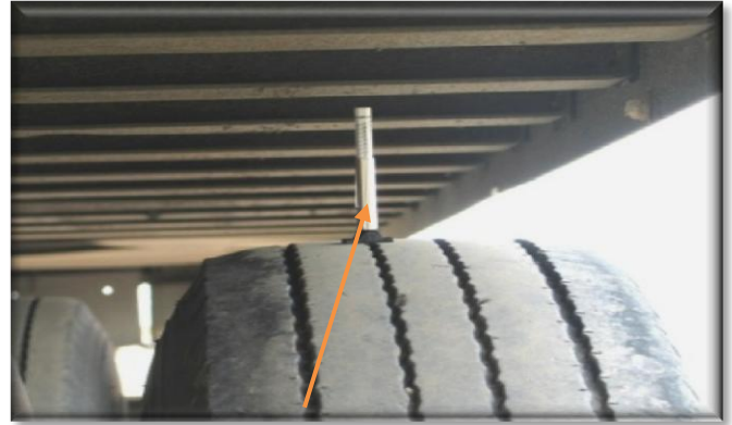
Checking Tread Depth and Inflation
