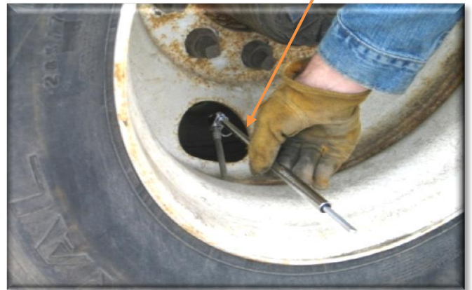
Checking Tread Depth and Inflation
